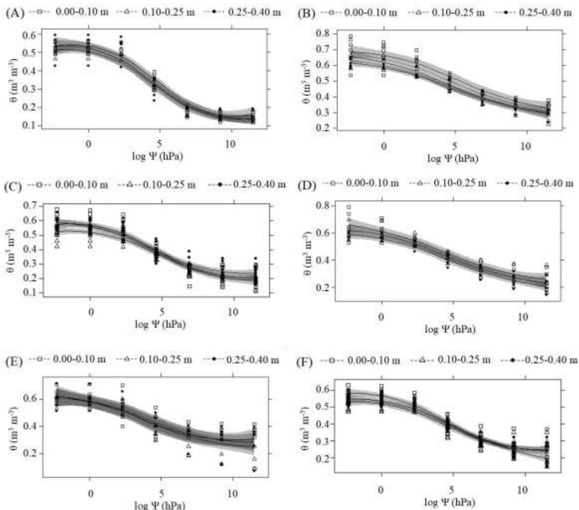
**Figure 8.** Soil water retention curve (SWRC) obtained with the Van Genuchten equation and parameters estimated with the SPLINTEX pedotransfer program in localities of Subtropical region of Brazil: (A) Arapoti; (B) Castro; (C) Ponta Grossa; (D) Socavão; (E) Tibagi; and, (F) Itaberá.
