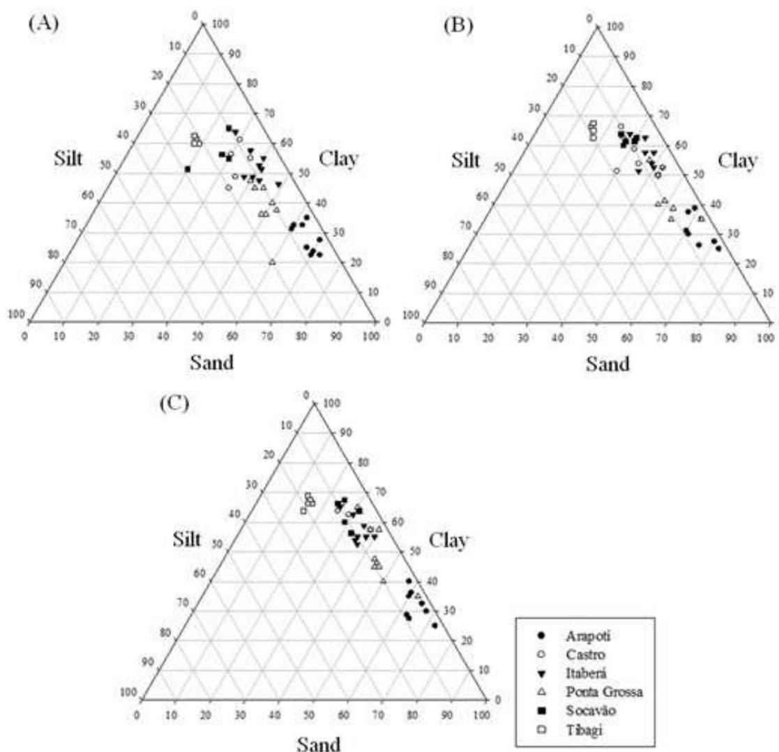
**Figure 2.** Granulometric distribution of the soil samples collected in the layers: (A) 0.0 - 0.10 m; (B) 0.10 - 0.25 m; and, (C) 0.25 - 0.40 m, from no-tillage systems in the localities of Arapoti, Castro, Ponta Grossa, Socavão and Tibagi - Paraná, and Itaberá - São Paulo, Subtropical region of Brazil.
