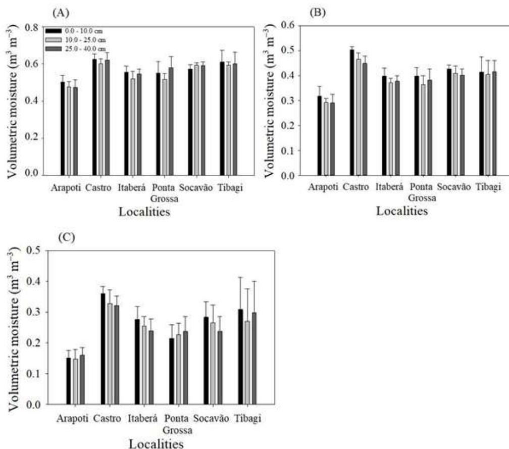
**Figure 5.** Soil volumetric moisture at saturation ( $\theta_{sat}$ ; A), field capacity ( $\theta_{FC}$ ; B) and permanent wilting points ( $\theta_{PWP}$ ; C) of samples collected in no-tillage systems in the localities of Arapoti, Castro, Ponta Grossa, Socavão, and Tibagi - Paraná State, and Itaberá - São Paulo State, Subtropical region of Brazil.
