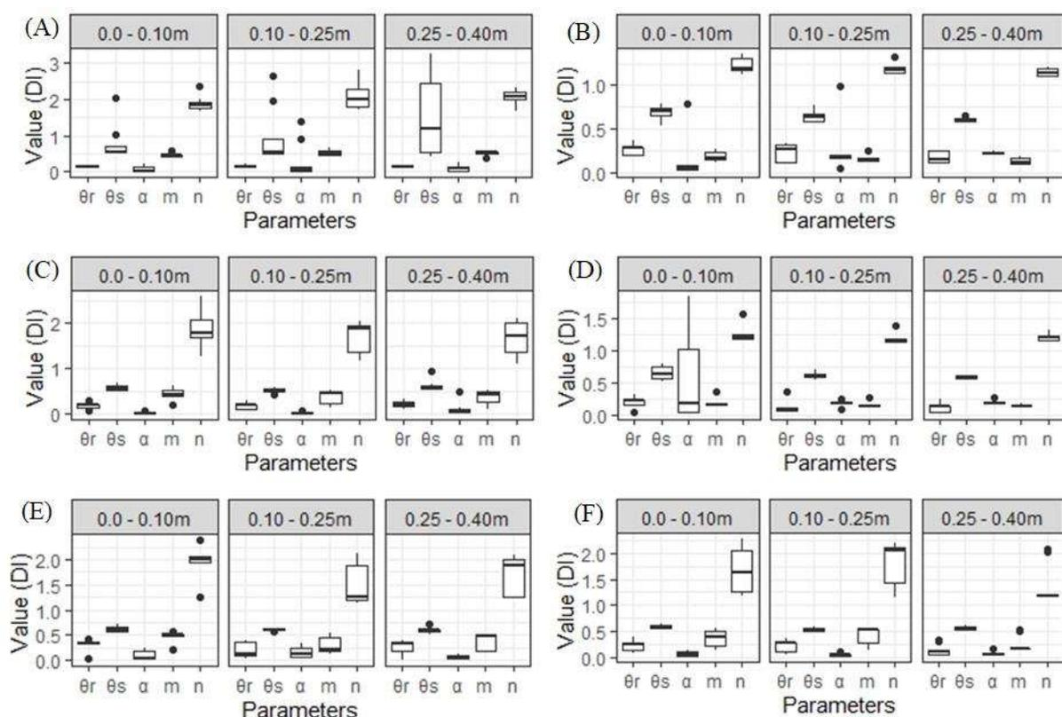
**Figure 7.** Parameters of the Van Genuchten equation obtained with the *SPLINTEX* pedotransfer program in the localities of Subtropical region of Brazil: (A) Arapoti; (B) Castro; (C) Ponta Grossa; (D) Socavão; (E) Tibagi; and, (F) Itaberá.
